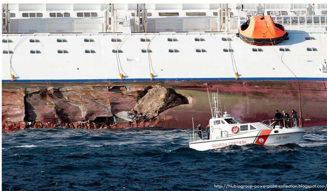
Giglio, Italy — Rocks are visible in the damaged hull the Costa Concordia. PHOTOGRAPH BY: Gregorio Borgia / Associated Press
